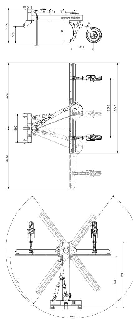
Weight 305 Height of the blade: Rotation of the main blade's edge Total boom length The main width of the blade The maximum swing angle boom The max. swing distance from center Wheel dimension Air pressure Wheel dimension Air pressure 600 kg w/hydraulics and wheels 700 mm 286 degrees 2120 mm 3050 mm. 25/20 degrees with hydraulics 2290/2170 mm with HTS 305 5.00 x 8 6- layer Max 75 lbs or 525 kpa (5,2 bar) 6.00 x 9 10- layer Max 101,5 lbs or 700kpa (7 bar)
